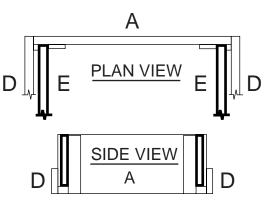
Push the "END BARS" into the gap as shown. Attach the TOP BARS. Flip the jig over and attach the BOTTOM BARS. To remove the frames from the jig, pull up the end supports (F) and remove the inner support. Replace the inner supports, load up the end bars and make another perfect batch!
